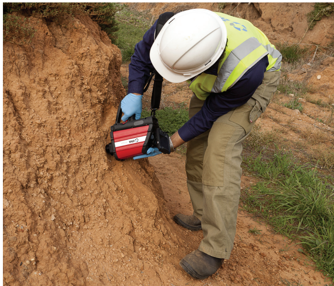
The RemScan™ device uses an infrared signal to directly measure petroleum contamination in soil.
