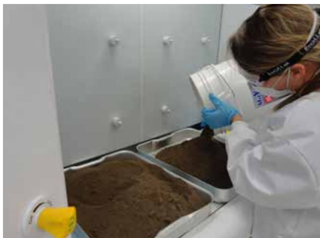
Preparing soils for RemBind treatment
