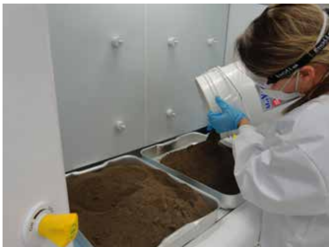
Preparing soils for RemBind treatment
