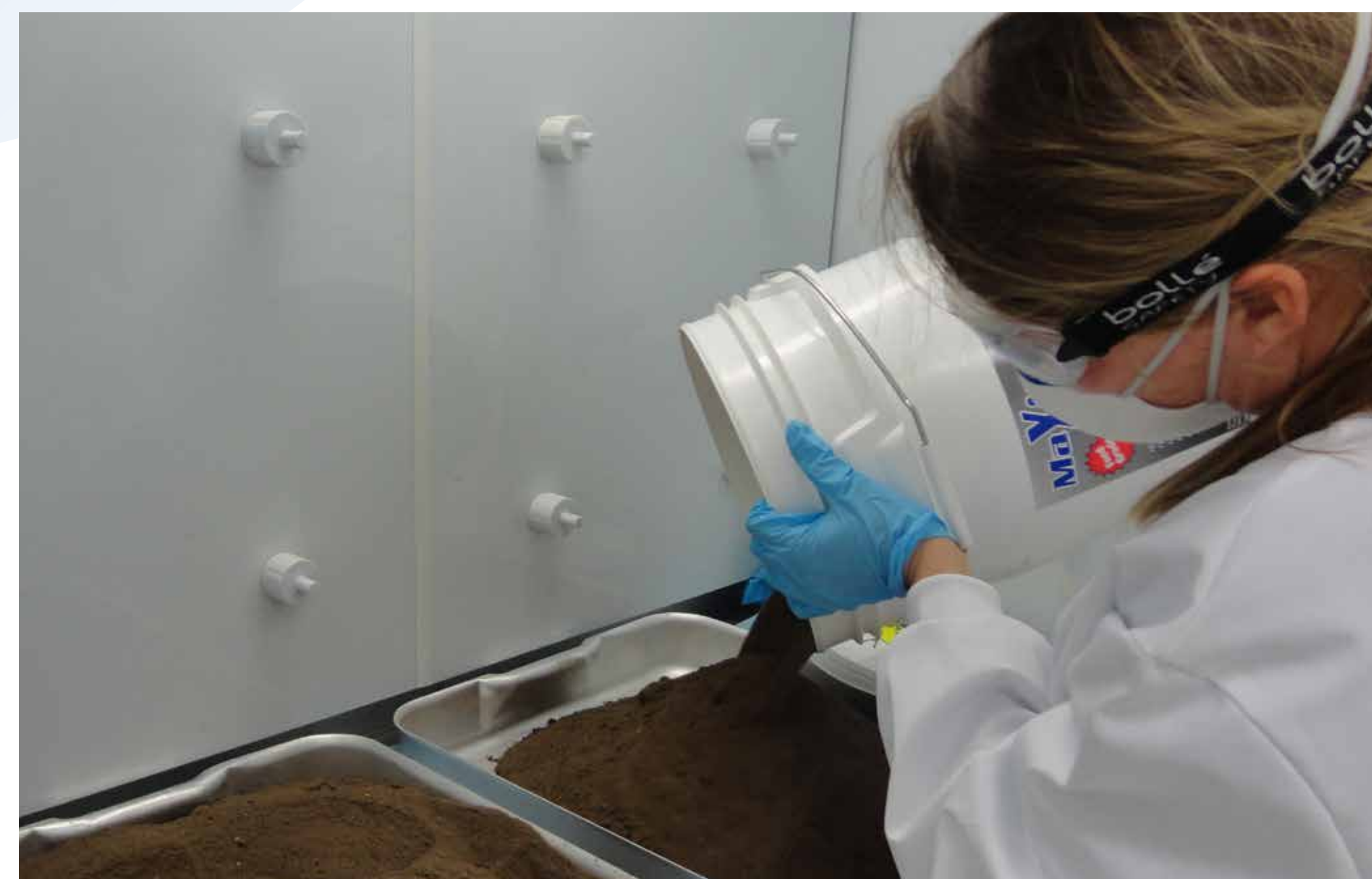
Figure 2: Preparing AFFF-contaminated soil for the addition of RemBind and RemBind Plus
