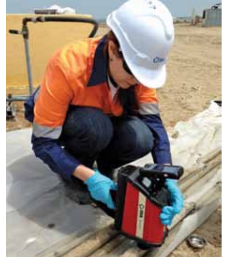
Using RemScan as a screening tool at Site 2.
